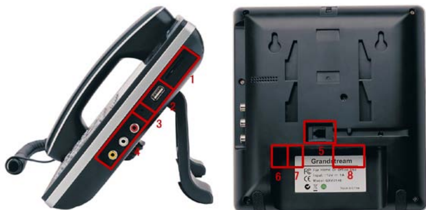
Figure 2: Connecting the GXV3140
